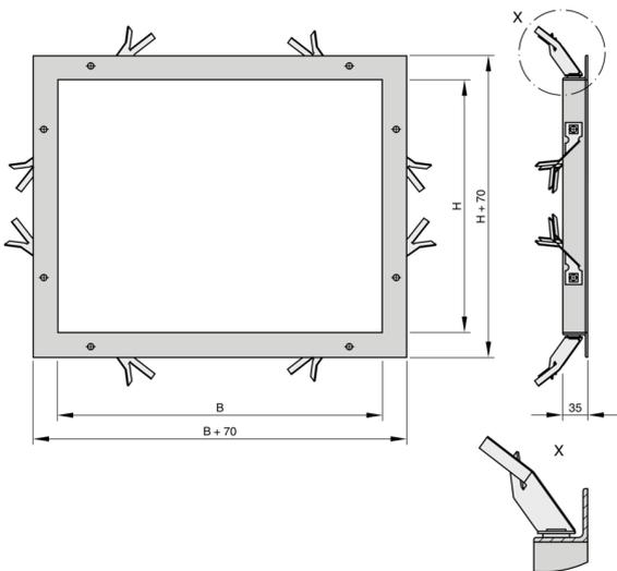
Before the subframe is mortared in, the fixing tabs must be bent and spread (by others).
