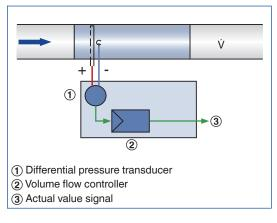
available as a voltage signal. The factory setting is such that 10 V DC always corresponds to the nominal volume flow rate ( $\dot{V}_{nom}$ ). Voltage ranges are factory stored in the controller. Changes on the customer's site can easily be carried out using an adjustment device or a notebook with service tool.
