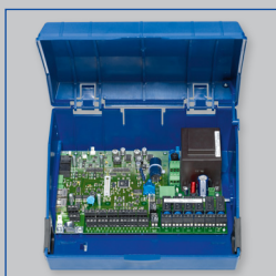
EASYLAB adapter module TAM
