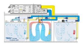
Taking into account the diverse, varying requirements in laboratories, a concept was developed that integrates all important functions in one complete system: the TROX UBox. It can respond to different conditions with real demand-based ventilation and air conditioning, dissipate thermal loads in an energy-efficient manner and take into
